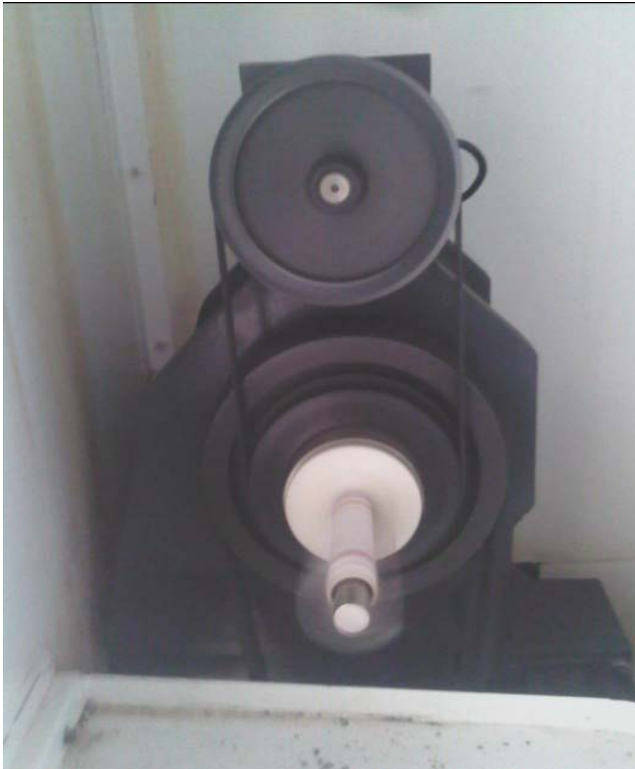
Figure 5 AC motor: 7.5KW
